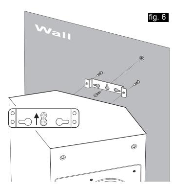
the cabinets' shape to aim the speakers inward toward the listening position. If the VS-2a's are to be mounted on the rear wall of the room, it is advisible to mount them horizontally and high up on the wall, using the cabinets' shape to aim the speakers downward toward the listening position.
